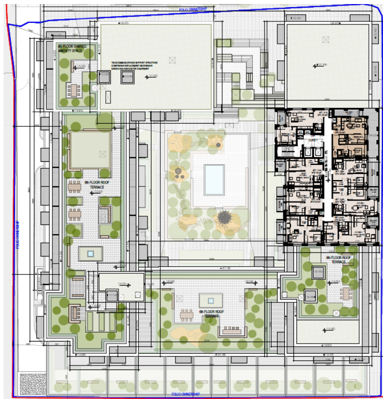
Figure 38.0 Fourteenth floor plan. 7 no. one-bedroom apartments and 1 no. two-bedroom apartment are provided at this level.
