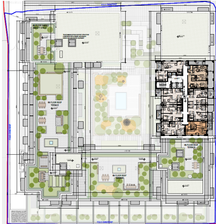
Figure 40.0 Sixteenth floor plan. 1 no. one-bedroom apartment and 7 no. two-bedroom apartments are provided at this level.
