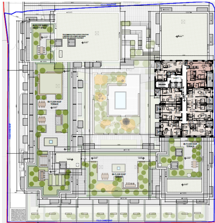
Figure 36.0 Twelfth floor plan. 7 no. one-bedroom apartments and 1 no. two-bedroom apartment are provided at this level.
