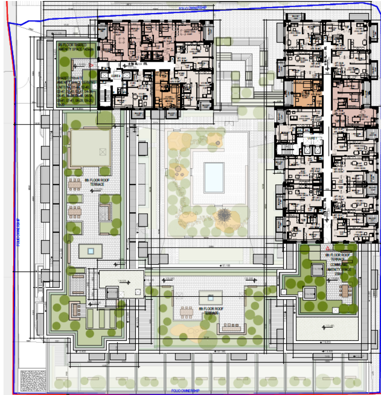
Figure 33.0 Ninth floor plan. We note the provision of a communal roof terrace at this level and a shared private roof terrace for the 15 no. units not served by private amenity space. 2 no. studio apartments, 15 no. one-bedroom apartments and 3 no. two-bedroom apartments are provided at this level.
